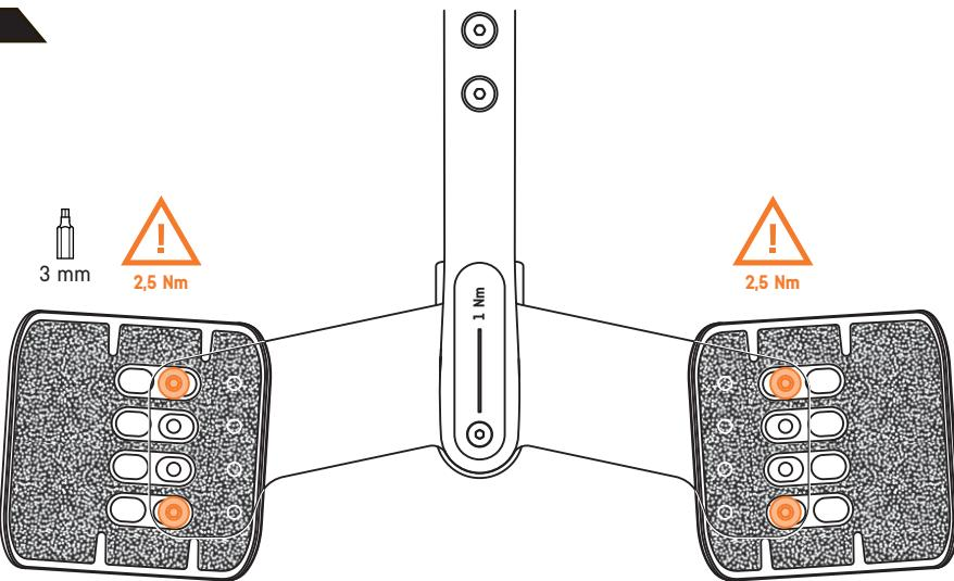
ALWAYS USE TWO SCREWS PER ARMSHELL AND MAKE SURE THEY ARE ALWAYS IN THE SAME VERTICAL ROW. THEY CAN BE MOUNTED ON TOP OF THE OTHER WITHOUT ANY DISTANCE, OR WITH A GAP OF ONE OR TWO HOLES.
