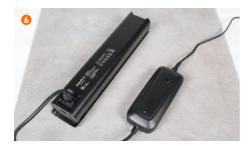
Now you can charge the removed battery with the charger supplied (6).
