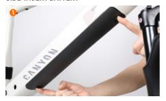
If your Canyon is equipped with a side-insert battery, you can either remove the battery for charging or charge it while it is mounted.
