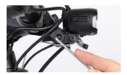
Use a 3 mm Allen key to loosen the fixing screw of the front light just as far as necessary to move the front light up and down in the holder by hand
