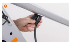
Then insert the charging plug of the supplied charger into the charging socket (8).
