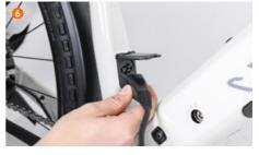
Then insert the charging plug of the supplied charger into the charging socket (6).
