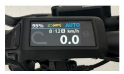
The display shows information about the shifting, e.g. the chosen shifting mode and the gear engaged.
