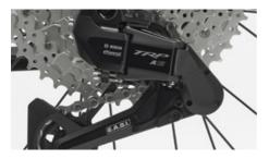
The automatic TRP shifting system shifts and changes gears during the ride.
