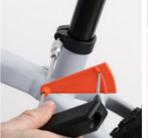
Slowly turn the handle of the Canyon torque wrench. When the bolt is tightened, the pointer moves over the scale. Stop the turning movement as soon as the pointer reaches the marking of the prescribed torque value.
