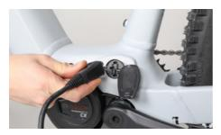
Insert the charging plug of the supplied charger into the charging socket.
