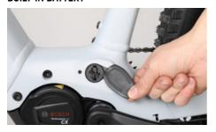
Open the cover of the charging socket above the bottom bracket.
