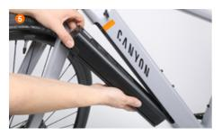
Remove the battery from the lower holder in the down tube (5).
