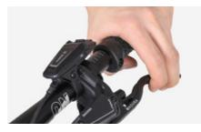
The ABS is activated automatically when you activate the brakes. It is crucial that you use the brakes as you are used to. Don't be put off by the fact that the brake or brake lever jerks a little, especially at the course of the braking process. The ABS system is only activated if you keep the brake lever pulled.
