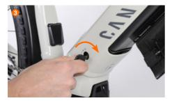
To **remove the battery** you have to unlock the battery with the key **(3)**.
