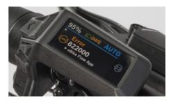
If the LED does not light up when the drive system is switched on or does not go out when the speed reaches 5 km/h (3.1 mph) or lights up continuously during the ride, the ABS is defective.
