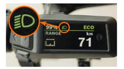
The light has to be activated on the display. Depending on the model and software, this may be done automatically as soon as the system is switched on.
