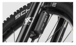
Some models, such as the Pathlite:ON SUV and Grand Canyon:ON are equipped with Bosch's anti-lock braking system (ABS).
