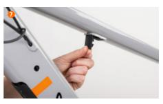
To charge the battery while mounted open the cover on the top tube first (7).
