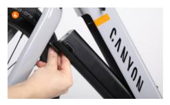
Continue holding the battery in place. Slowly tilt the battery downwards (4).
