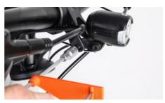
Once you have set the correct position, tighten the fastening screw of the light to 3 Nm.
