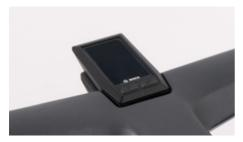
Some models with Bosch drive are equipped with a KIOX display. This display is held in place by magnets.
