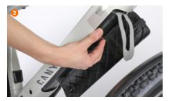
Now you can fold up the cover towards the side. From now on hold the battery in place with one hand (2).
