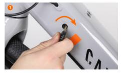
To remove the battery you have to unlock the battery with the key (1).
