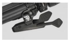
You have got the option to manually overrule the automatic shifting for 10 seconds. I.e. you can adjust your gear manually at any time.
