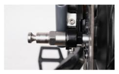
For e-bike models with a hub gear, it is not necessary to replace the complete axle to be able to use the Croozer trailer. All need to do is replace the axle nut on the left-hand axle side.
