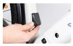
To charge the **battery while mounted** open the cover above the bottom bracket first **(5)**.
