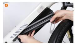
Reach into the grey tab at the top end of the battery and remove the battery downwards from the mounting (4).
